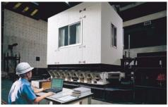
Life-size mockup at structural testing site that verifies seismic
