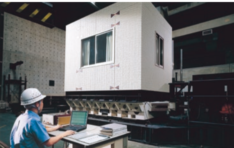
Life-size mockup at structural testing site that verifies seismic resistance levels
