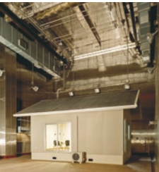
Test in an artificial climate room to verify insulation and comfort
