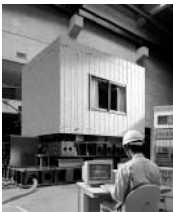
Vibration test of full-scale exterior wall
