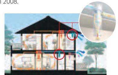
Amenity Ventilation System II The cyclone unit and high-performance filter supply clean air to indoor spaces.
