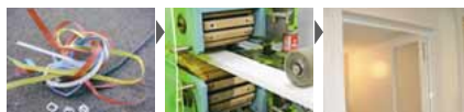
Waste packaging materials are used in bathroom entrance frames in Sha-Maison rental apartments.
