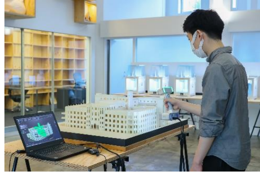
Digital archiving of architectural models with a 3D scanner
