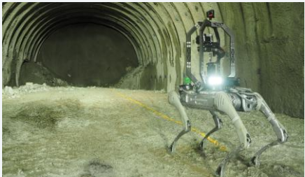
Quadruped on-site inspection robot “KOCORo”
