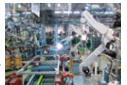
Automated production lines that can produce a wide range of housing frames entirely on a customer-distinctive basis (Shizuoka Factory)
