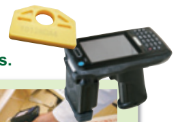
4 IC tags are scanned with a dedicated device according to the category.
