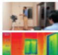
Testing to validate heat insulation effect is conducted in an artificial weather control room.
