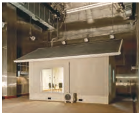
Test carried out in an artificial climate room to verify insulation and comfort
