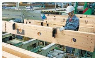
To reduce the workload at construction sites, metal fittings are pre-attached to structural frames, which have been precisely pre-cut via computer control
