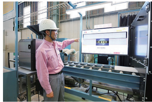
AI-based quality management system for Bellburn earthenware wall panels
