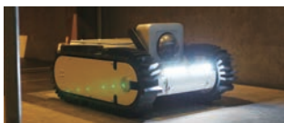
Underfloor inspection robot
