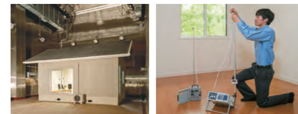
Test carried out in an artificial climate room to verify insulation and comfort
