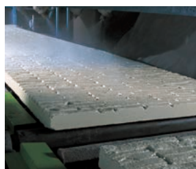
Coating line for Dyne Concrete applies 4 layers of coating to enhance durability and weatherability
