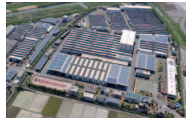
Installing mega-solar power systems at our 5 factories nationwide for a total of 6.7 MW
