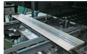
A sensor camera is used to check the size, color tone, and gloss of Bellburn tiles, which are customized for each customer
