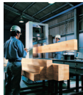
A SHAWOOD house beam is tested for flexural strength as part of strict quality control at our factories
