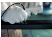
Inspecting the thickness of anti-rust coating on steel frames
