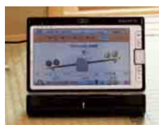
The amount of power produced can be checked daily on the display of the CO 2 monitor. (The monitoring is conducted as part of the 2008 Model Project for Reducing CO 2 in Residential Buildings.)
