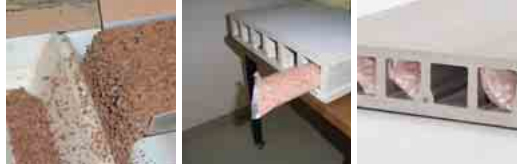
Particles of finely pulverized waste roof tiles are used as filling materials to absorb vibrations.
