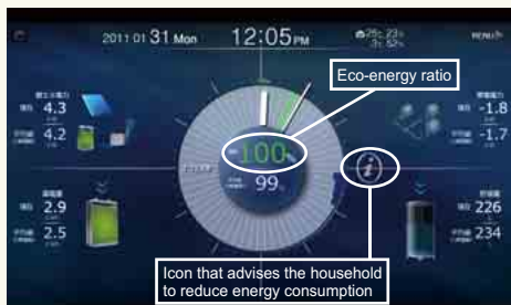
◀HEMS display (example) The display shows the energy information of the household such as the amounts of electricity generated, stored and purchased; amount of hot water in storage;
