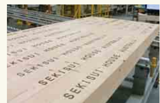
A factory was opened in the vicinity of the Camden Hills construction site to precut timbers.
