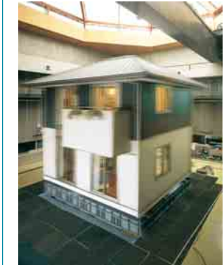
We became the first Japanese housing manufacturer to conduct earthquake-resistance testing using an actual sized home in 1979. Our continued testing and validation efforts led us to the development of advanced seismic solutions such as seismic-isolated and seismic-dampening structures.
